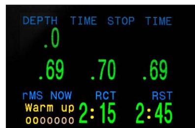
So this will become a new rule when using the scrubber monitoring system: always pre-breathe until you have at least 45 minutes CYCLE time (green): this means that the scrubber is
