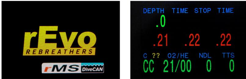
If you don't see the C ??, then the scrubber monitoring system is not activated. To activate the system, go to System Setup+, where you will find a new page 'rMS Setup'
