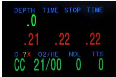
This tells you that the exhale scrubber communicates with the system, but there is no communication with the temp probe of the inhale scrubber. At this moment, you can even check the temperatures in the scrubbers: at the Scrubber+ screen, pushing the correct right buttons gives you:
