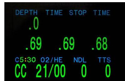
Also on the main screen there is an indication if the scrubber is fully ready or not: as long as the warming up is not yet finished, the colon between the C and the number is yellow, and only when the scrubber is fully warmed and ready, the colon becomes green, and full information of the total scrubber can be used to predict the cycle and scrubber times.
