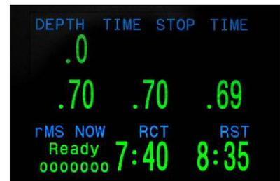
From this point on, and in dive mode, the minimum remaining cycle and scrubber time of the dive is logged, while at the same time the actual RCT/RST is shown on the main screen and the extra info screen.
