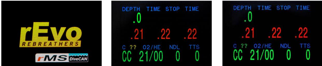
If you don't see 'C ??' this means that your temperature probes are switched off in the 'rMS Setup'. Go to the setup menu and change the setting of the temp probes to 'on'. Switching 'off' the temperature probes can be done when diving on the dual radial scrubbers, or when using classic non-rMS axial scrubbers.
