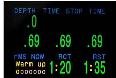
With only the temperature info at the inlet of the scrubber, the system has already received enough data to predict a minimum remaining time. You can see on the info screen that the warming up of the first zone in the scrubber has started: the color changed to yellow.
