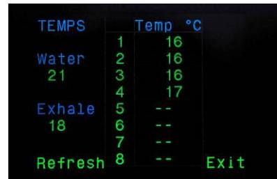
You notice that the temperatures of the first scrubber, the top scrubber, are indicated (temp 1 to 4), but that there is no indication of temperature 5 to 8: the sensors of the temperature probe in the inhale scrubber.
