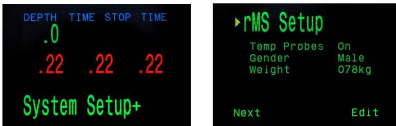
The rMS setup screen allows you to turn on and off the temperature probes, so switching on and off the scrubber monitoring system.
