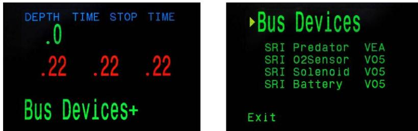
A right push on Bus Devices+ will show you all the devices connected to the CAN bus, and the software version they are using. This screen allows you to easily identify if one of the devices is missing, and if you are using the correct software in each device.
