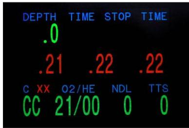
The two red XX show you that there is no communication with either of the temp probes. If communication with one of the temperature probes is successful, you see:
