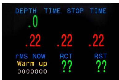
This screen shows that the unit is ready for warm up, but none of the 7 zone's in the scrubber have started to become active (they are all grey) so no prediction can be made for RCT or RST
