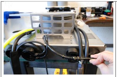
Now we install the upper cable from the battery box to the exhale lung.
