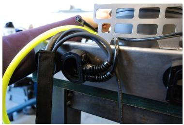
... makes a gentle curve toward the entry port. The excess cable is pushed into the port. Now fasten the second screw of the cable gland: hand tight and then only ¼ turn with a key or pliers. There should be +/-1mm to 1.5mm between the 2 parts of the cable gland.
