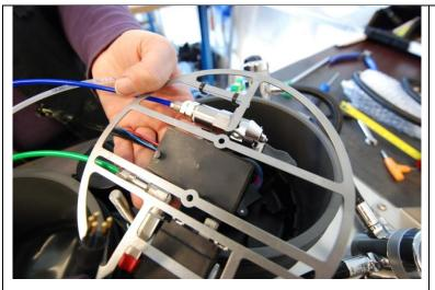
When holding the tray this way, the blue and green hose should make a nice curve towards the exhale lung
