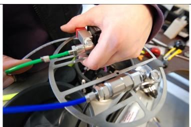
When you push the tubes on the connectors, green on the solenoid, and blue on the ADV, make sure that you push the hose completely over the barb, without kinking the tube, fasten the tube gland manually as far as you can...
