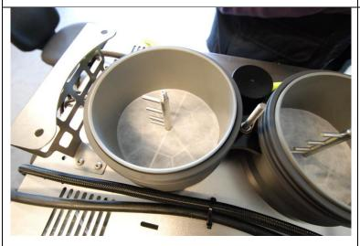
Now the rMS canisters must fit gently inside the scrubber holders, while the temperature probes touch the center of the solenoid- and oxygen board;
