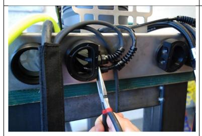
.. use a key or pliers to screw the gland till the end.
