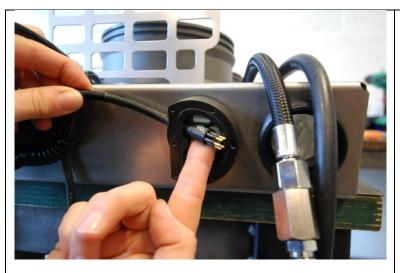
Bent the connector gently outwards, and pull the cable to the outside of the unit.
