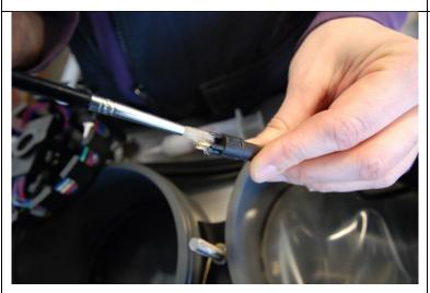
Before plugging the DIVECAN connector, lubricate a little bit with silicon oil.
