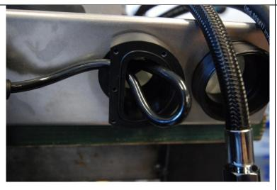
Push the cable in the upper opening till you have a small part left, and then pull on both sides of the cable, outside the unit,...
