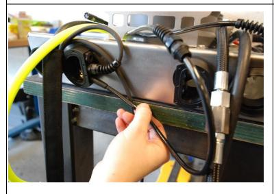
The middle cable goes to the bottom hole in the triple connector. The middle hole is for the first rEvodream, and the upper hole is for the optional second rEvodream
