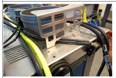
Slide the middle and the upper cable, with the male connectors, under the top protection of the rEvo
