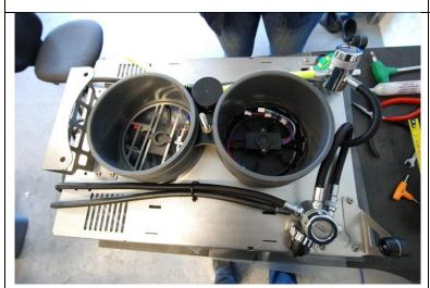
When you insert the solenoid grid in the exhale lung, the tubes and the cables make a nice turn so that they are not located under the tray;
