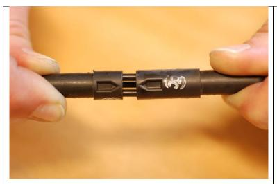
Then push the connector till the end. (the picture shows when it is not yet fully connected)
