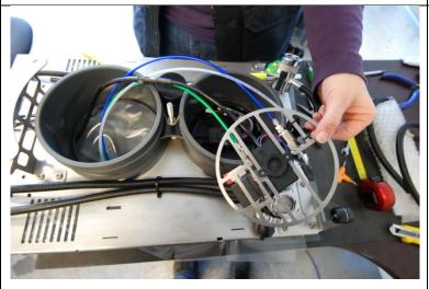
... and connect the DIVECAN cable of the solenoid board with the cable in the exhale lung, using a bit of silicon oil;
