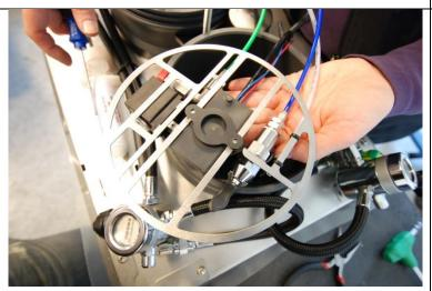
... fasten the solenoid board with the threaded plastic part.
