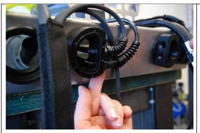
Screw the first part of the cable gland into the triple connector, and..
