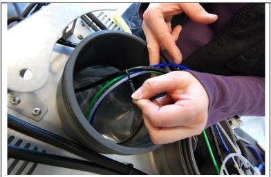
Use a tie wrap to fasten the 3 tubes and the DIVECAN cable together, and push the tie wrap as far as possible inside the exhale lung, over the tubes.
