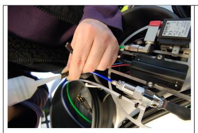
To prevent corrosion of the electrical connectors of the solenoid, you can put some oxygen compatible grease inside the cable connector.
