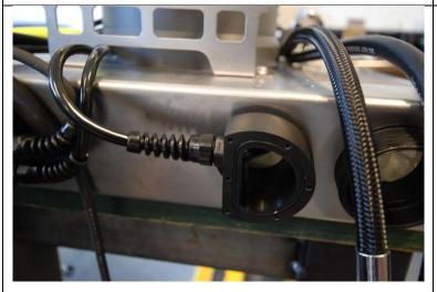
Adjust the length of the cable so that there is no stress on the cable, and the cable makes a nice curve towards the OPV.
