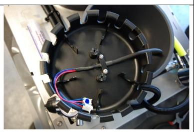
If the cable would 'slide' under the fixation, you can always fix a small tie wrap around the cable, that will prevent it from moving away.
