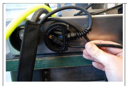
Put the male connector through the bottom hole ...
