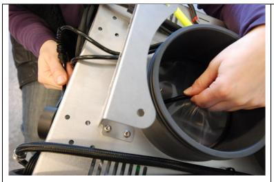
... and at the same time at the end of the cable inside the exhale lung, so that you try to 'rubb' the cable as little as possible against the walls of the OPV.
