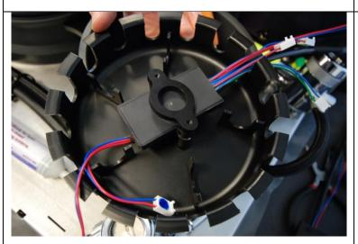
... and fasten the board with the threaded plastic part.
