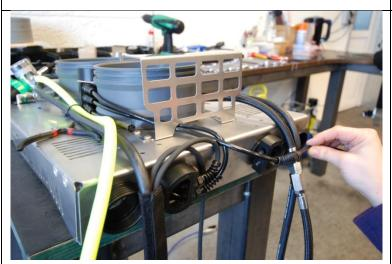
Make sure the cable does not make twists around other cables.
