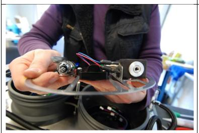
Now slide the electrical connectors over the pins of the solenoid..
