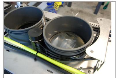
Put the battery pack in place. The lowest cable from the battery pack goes to the Predator Divecan.
