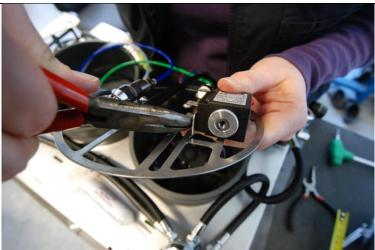
Use pliers to bend the lower connector of the solenoid, the one closest to the solenoid grid, a little bit up.
