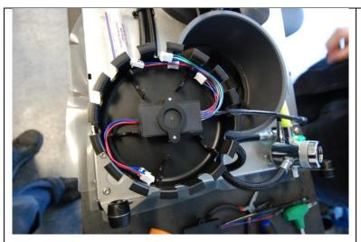
You will notice that the connectors of the sensors have different length, the shortest goes to cell fixation 1.
