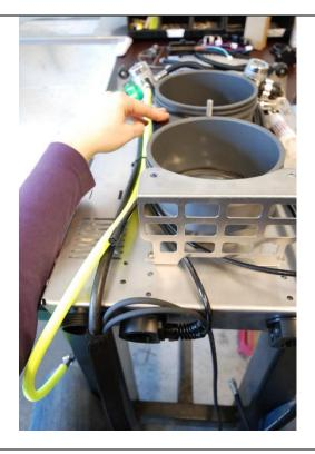
Now check for the correct length of the cable: the cable should make a nice route to the triple port, so that there is no stress on the cable, and ..
