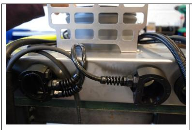
Fasten the second, the outer screw of the cable gland, hand tight and then ¼ turn with a key or pliers.
