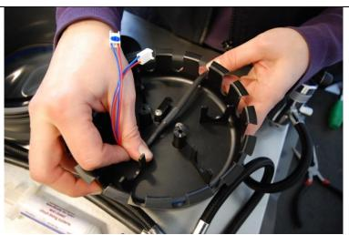
Before fitting the parts of the rMS, fasten the cable (s) of the rEvodream onto the new sensor tray.
