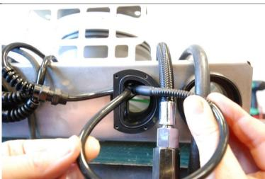
Now insert the cable in the UPPER SMALL opening of the OPV port: the cable should NOT go into the main bigger opening, as that opening is reserved for the functioning of the OPV itself.
