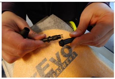
For the DIVECAN connection outside the unit, we use a security clip that holds the connector together, preventing accidental disconnection, but that allows disconnection only when the cable is subjected to a hard 'pull', so that the cable is protected against damage. Put the 2 O-rings over each connector,...
