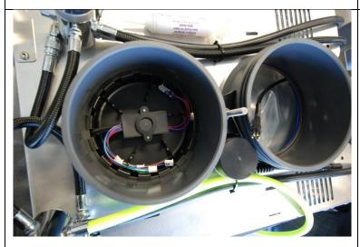
When installing the sensor tray under the inhale scrubber, make sure the DIVECAN cable, and the rEvodream cable make a nice curve in the lung, so that they are not under the sensor tray.
