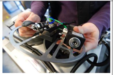
This way the cable that feeds the solenoid can just pass the solenoid board.
