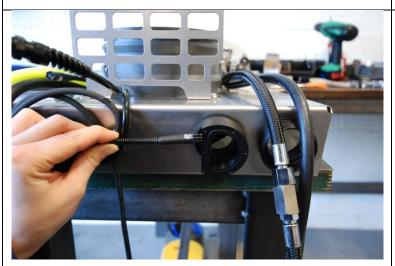
Insert the cable into the upper hole of the OPV.
