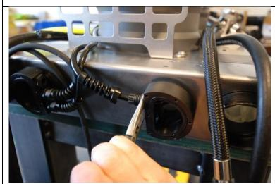
Fasten the first screw of the cable gland.
