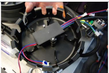
....put them through the oxygen sensor board of the rMS, (remember the CAN cable with the connector on the same side as where the rEvodream cable comes in)..
